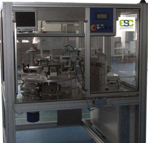
The GRINDING & BRUSHING Machine GRD-BR-4 made by ESC allows grind and brush the needles at the end of the assembly process.
