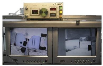
The laser system is a cutting edge diode laser source together with an high tech welding head focusing the 975 nanometer laser beam to the right position to get the best brazed joint.
