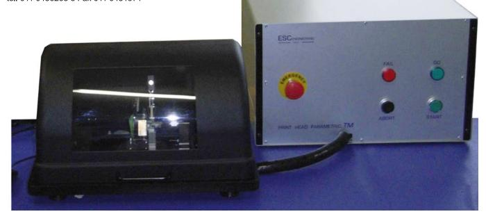
The Print Head Parametric Testing Machine made by ESC allows to measure the main working parameters of dot matrix print head.
